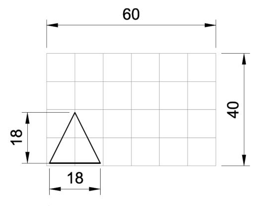
Calculate the amount of material wasted when producing the shapes you have drawn Assume no material is wasted when cutting.
