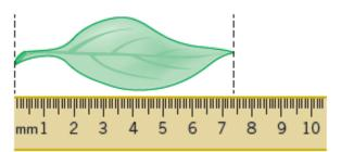
Using a ruler with a mm scale, the length of the leaf seems to be 74 mm. The smallest division is 1 mm, so the uncertainty is 0.5 mm.
